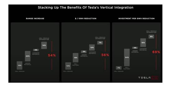
By experimenting with every component of its battery—from cell design, anode material, cathode material, to the process by which cells are placed into the vehicle, to even the design of the cell factory itself (!)—Tesla is working to achieve an astounding vehicle range increase of 54% while simultaneously decreasing the cost of produce thruput by 56% (i.e. expressed as \$/kWh of battery production).
