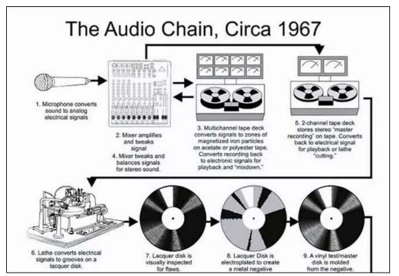
console (called a "lathe") to cut grooves into a vinyl record that create the sounds on the tape.
